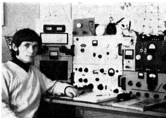
This outstanding 160 station, OK1ATP/Jardey, is in the forefront of dx working from Europe. The 1-8-21MHz, 10-80W home-built rig includes a 15-valve receiver and a three-valve converter. Photo via W1BB
